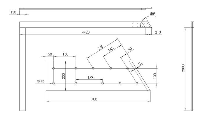
Supports of the lags of the floor and the lags of the second floor are ordinary boards of coniferous trees. Fixing lining are made of PSF plywood thickness of 20 mm. We recommend to leave a sufficient second light to organize the stairs and maximum aesthetics of the construction.
