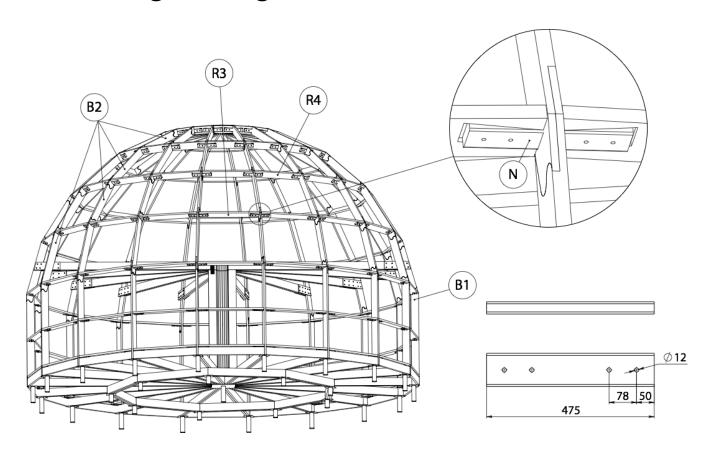
Drill through the nagel and the brace. The holes and their location are shown in the figure. Fix the brace and the nagel with a bolt M12 bolt with a nut and wide washers on both sides. A total of 4 bolts per each nagel.
