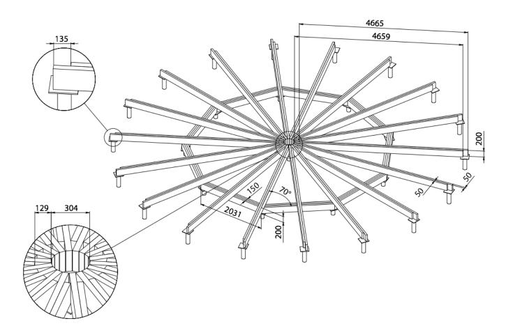
The lags of floor and the beams of foundation frame are not included in the delivery set, they are locally manufactured from dry lumber.
