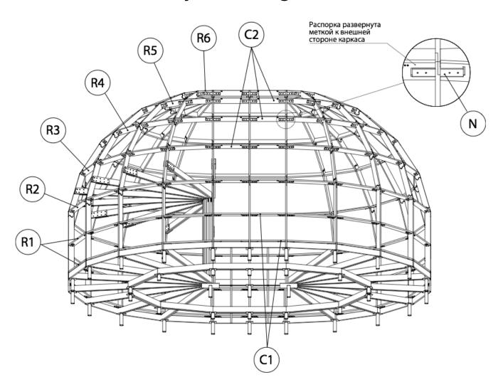
Drill through the nagel and the brace. The holes and their location are shown in the figure. Fix the brace and the nagel with a bolt M12 bolt with a nut and wide washers on both sides. A total of 4 bolts per each nagel.
