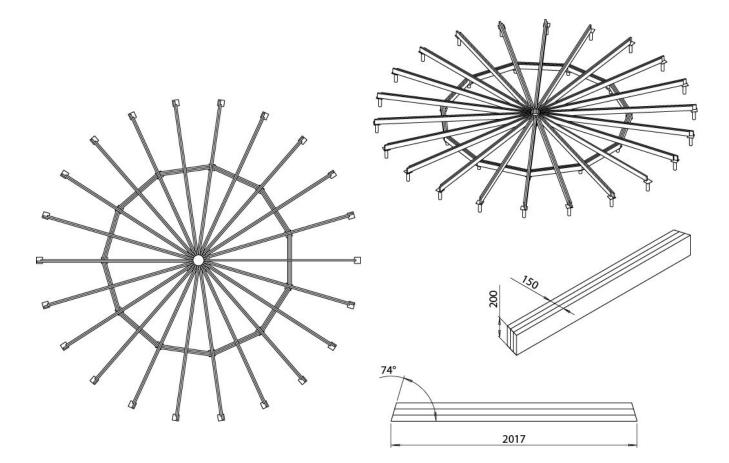
The beams of foundation frame are not included in the delivery set, they are locally manufactured from dry lumber.
