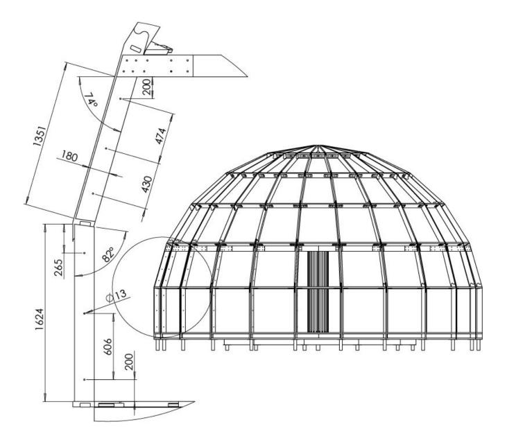
On the vertical beams to which the lags of the second floor are fixed, two boards are mounted - the amplifiers, the dimensions of which are indicated in the figure above. These boards are attached to vertical lags on 3 bolts each.
