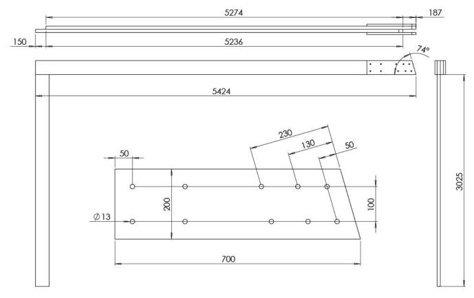
Supports of the lags of the floor and the lags of the second floor are ordinary boards of coniferous trees. Fixing lining are made of PSF plywood thickness of 20 mm. We recommend to leave a sufficient second light to organize the stairs and maximum aesthetics of the construction.
