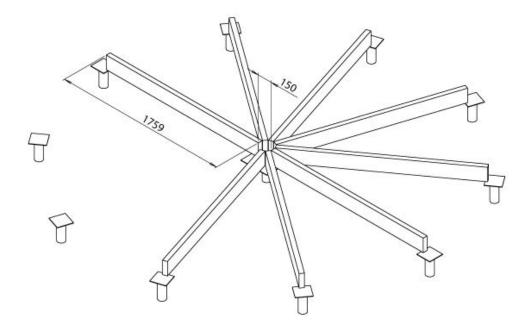
The lag of the floor is a regular board 150x50x1759 mm.
