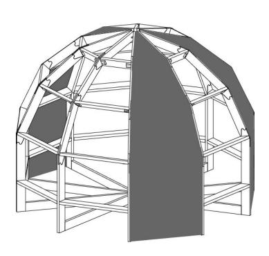
assembled horizontal tier. For the stability of the frame it is necessary to sew a minimum of three vertical sections of 10 - sew up from the bottom to the top.
