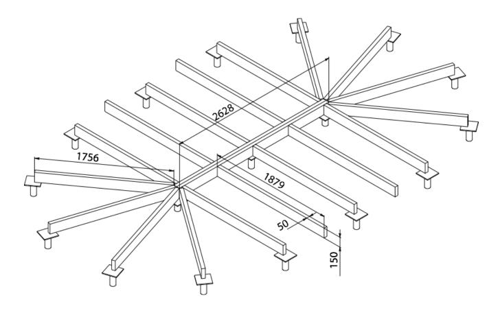
The lags of floor and the blocks of sheets are not included in the delivery set, they are locally manufactured from dry lumber.
