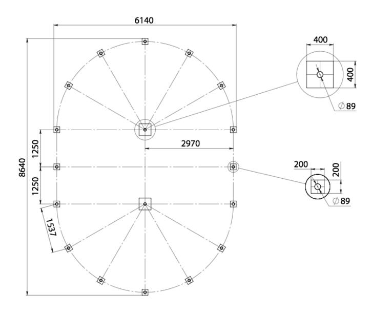
It is possible to use a band or monolithic foundation; combining of perimeter piles and concrete support in the center; other types of foundations.
