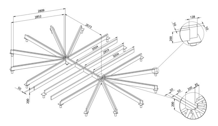
The lags of floor and the beams of foundation frame are not included in the delivery set, they are locally manufactured from dry lumber
