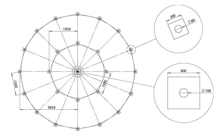
It is possible to use a band or monolithic foundation; combining of perimeter piles and concrete support in the center; other types of foundations.
