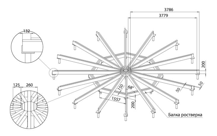
The lags of floor and the beams of foundation frame are not included in the delivery set, they are locally manufactured from dry lumber.
