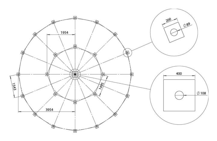
It is possible to use a band or monolithic foundation; combining of perimeter piles and concrete support in the center; other types of foundations.
