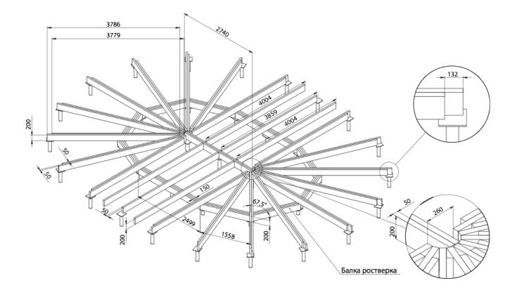
The lags of floor and the beams of foundation frame are not included in the delivery set, they are locally manufactured from dry lumber.
